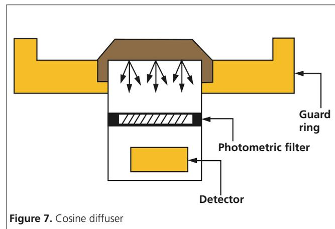
Figure 7. Cosine diffuser
