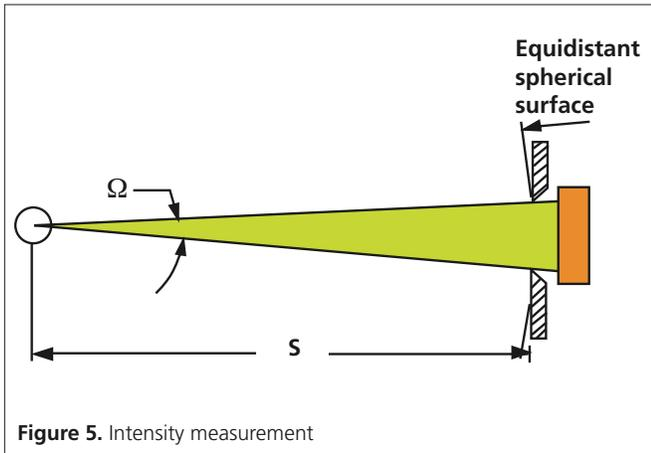
Figure 5. Intensity measurement
