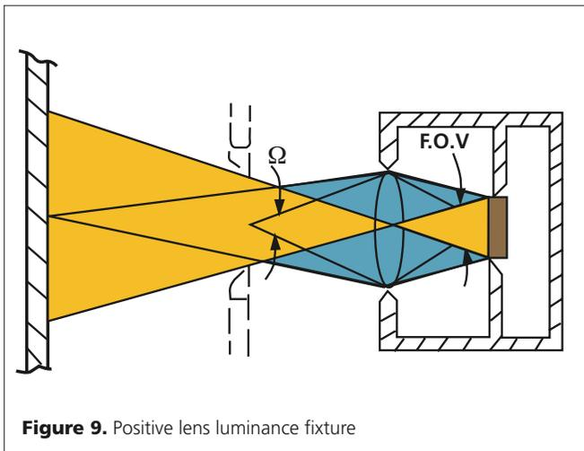
**Figure 9.** Positive lens luminance fixture
