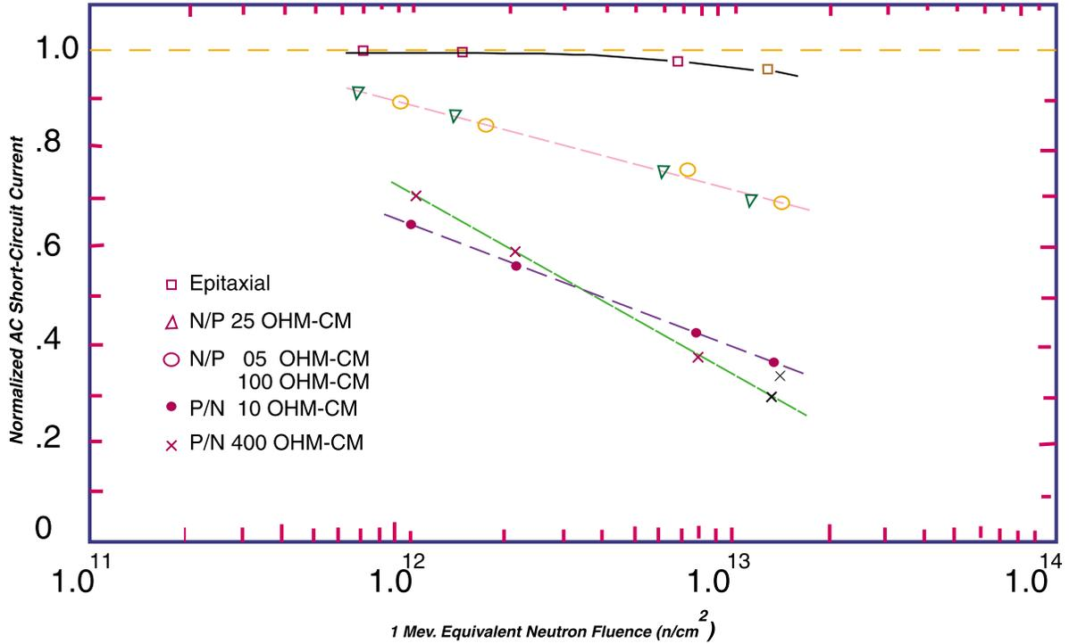
FIGURE 2. Photodiode AC short\_Circuit Current Versus Neutron Fluence
