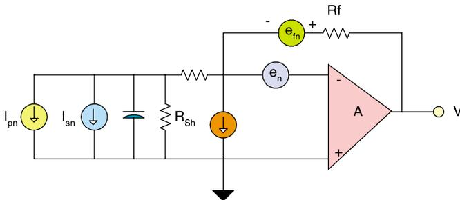
**Figure 5. Photodiode and Photodiode Preamplifier AC Equivalent Circuit With noise Source**
