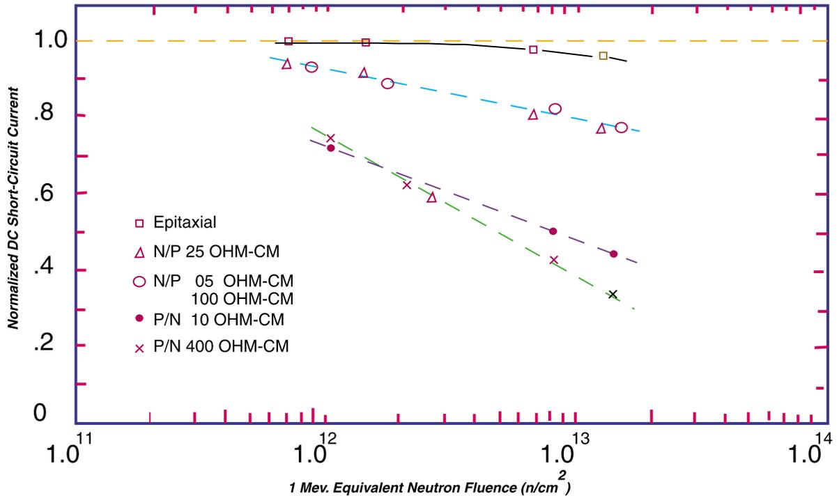
FIGURE 1. Photodiode DC short\_Circuit Current Versus Neutron Fluence
