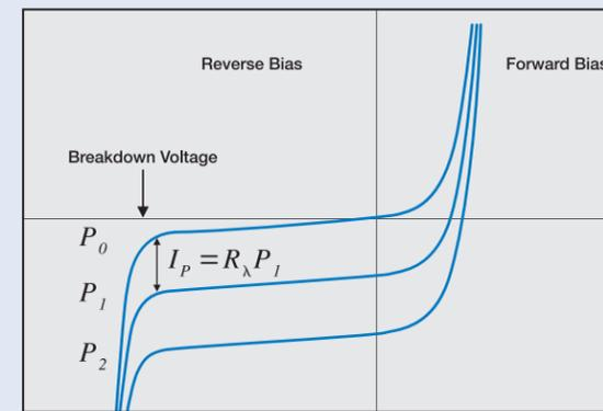
Figure 7. Characteristic I-V Curves of an OSI Optoelectronics photodiode for Photoconductive and Photovoltaic modes of operation. P<sub>0</sub>-P<sub>2</sub> represent different light levels.
