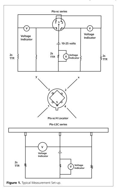
It is suggested that applications incorporate a back bias of at least 5 volts to get good linearity and responsivity. Increasing above this amount decreases unit capacity but does not increase responsivity or sensitivity significantly.
